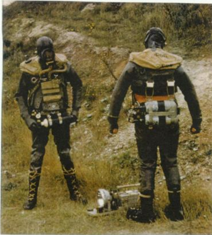
Siebe Gorman P-Party Sets (semi-closed circuit nitrox rebreathers) as modified for cave diving in the 1950s. L to R: Oliver Wells, John Buxton – photo taken by Tudor Johnston, March 31, 1957.
